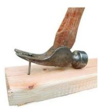
get the hammer positioned higher as in this illustration. This will give you added leverage.
