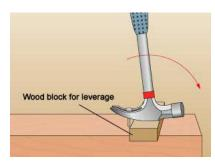
The claw portion of the hammer is slid under the nail head, and the handle is lifted up perpendicular to the surface by pulling from your biceps. Be careful, you can break the wooden handle or the hammer can slip and the force of your
