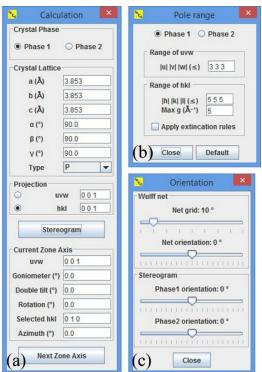
Figure 6. Three basic operational dialogs in SPICA4, (a) the calculation dialog, (b) the pole range dialog and (c) the orientation dialog for Wulff net and stereograms.
