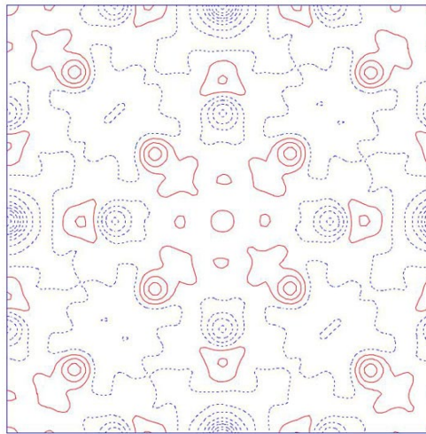
Figure 5. Atomic electrostatic potential difference map based on the diffraction data in Figure 4. The possible missing atoms are revealed in the dot line peaks.
